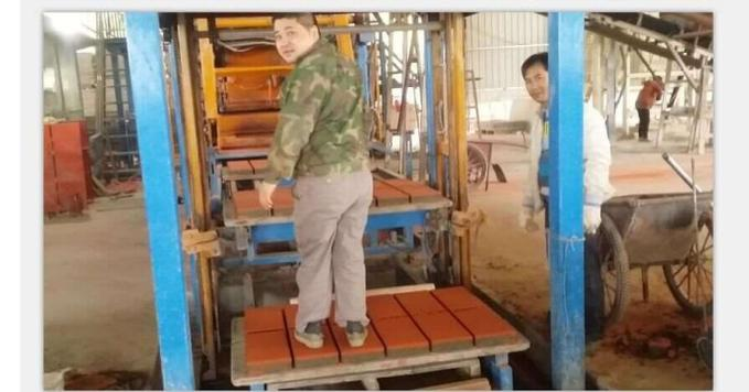
**3. Block Machine--**The mixed materials will be transferred to the block machine, After vibration and compaction of the mould, The fresh blocks will be produced.
