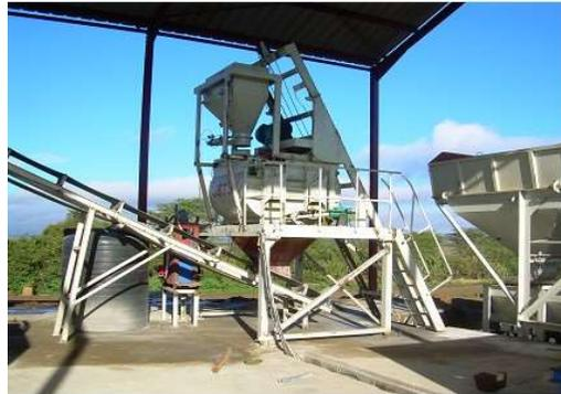
**2. Mixer---** the dosed materials will be lifted by the skip elevator to the mixer for mixing.
